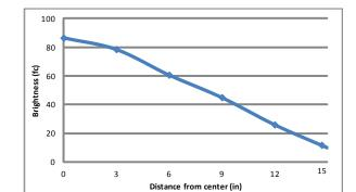
Photometrics: SF1-36 light source placed 18" away from work surface
