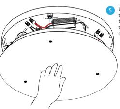
Use your hand to hold the canopy cover to the canopy, aligning the 3 holes to the 3 connectors.
