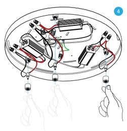
Connect the T-shape connectors to the LED driver by connecting the red and black wires to the LED driver respectively. Place it in the receiving holder in the canopy, and screw in Strain relief knobs to hold them in place.
