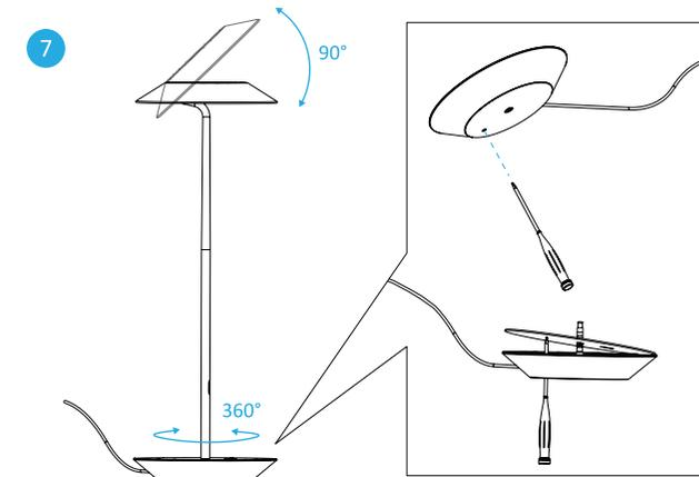
**Optional:** To change the cover plate, first unscrew the lamp body from the base, then use a screwdriver or any long and narrow object to poke through the hole at the bottom of the base and push the cover plate up. Repeat Step #2.
