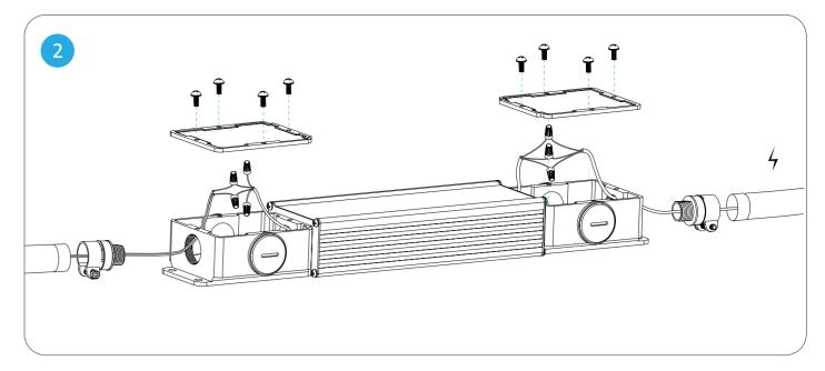
Using the provided DC cable & connectors, connect the wires inside the transformer enclosure as illustrated in the Wiring Diagram below. A transformer needs to be installed for every location marked with the symbol (
