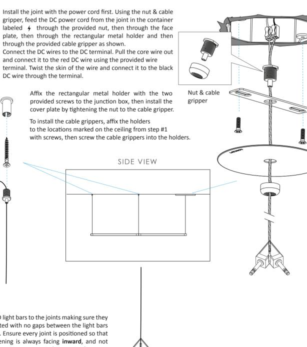
Attach the LED light bars to the joints making sure they are fully inserted with no gaps between the light bars and the joints. Ensure every joint is positioned so that its center opening is always facing inward, and not upward, downward or outward of the entire fixture.
