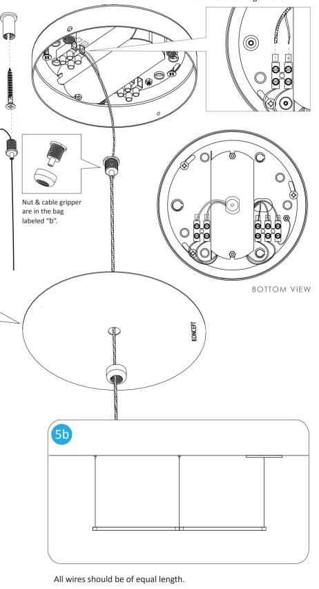
Wires can be released and re-adjusted by pressing the cable grippers' "nozzle".
