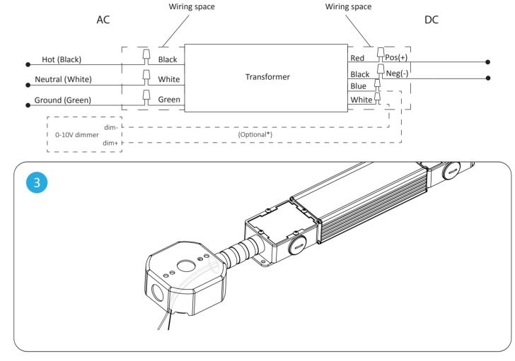
Feed the Red and Black DC wires through the conduit into the junction box (conduit and junction box not provided). Affix the transformer enclosure and junction box properly inside the ceiling, with an opening allowing access to the junction box.
