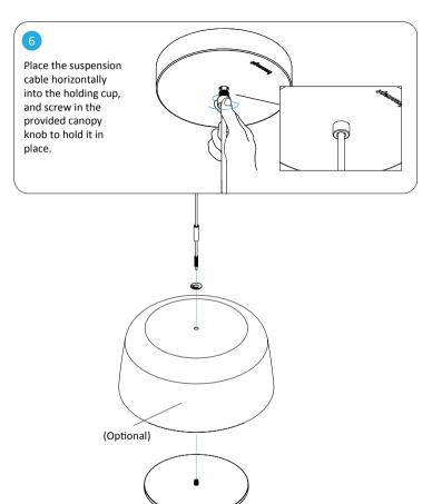
7 Connect the cable to the pendant head.
