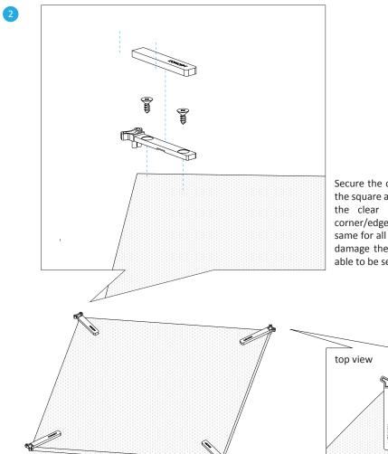
Secure the clear plastic holder with screws to a corner of the square acoustic panel. Make sure the protruding part of the clear plastic holder is sitting tight against the corner/edge of the rectangle acoustic panel. Repeat the same for all 4 holders. Be sure not to overscrew as it might damage the acoustic panel and the screws would not be able to be securely mounted.
