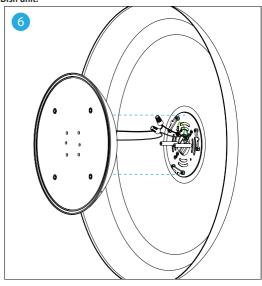
Insert the Ramen wall sconce onto the backplate on the wall by aligning the slots. Align the slots where the red dots are.
